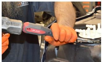
(Fig. 5) Loosen the OEM hold-down ring by turning it counter-clockwise.
