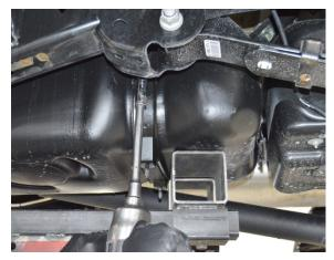
(Fig. 4) Remove OEM straps.
