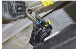
(Fig. 1) Remove OEM shield.
