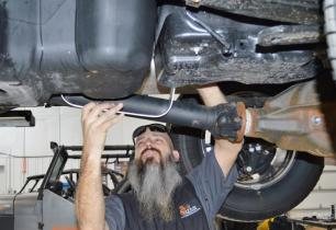
(Fig. 11) To install the new straps, turn and hook on inboard side of the tank, then rotate. Then tighten bolts on the outboard side.
