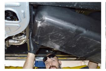
(Fig. 10) Angle tank slightly as it is lifted in so that front protrusion on tank slides over cross-member.
