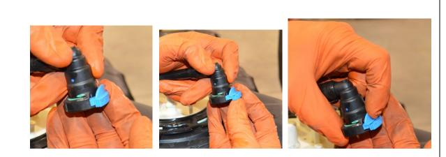
(Fig. 3): **Method for Disconnecting Fuel Line Couplings:** The couplings involved in this installation are of the quick connect type shown in left photo above. To disconnect, a) Slide the tab that has teeth on its edge outwards as shown in the center photo. b) Next, press the rounded button, as shown in the right photo, and pull the coupling apart.
