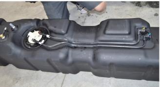
(Fig. 8) Use the OEM hold-down ring and tighten (Fig. 9) Fuel lines installed on the new TITAN tank. it by turning it clockwise as far as it will go.
