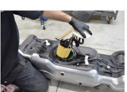
(Fig. 6) Remove the sending unit.
